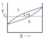
Which one of the following figures qualitatively represents the G-X (Gibbs free energy – composition) plot at temperature  $T_0$  shown in the phase diagram?
