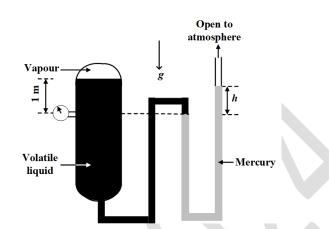
The height, h (in m, rounded off to two decimal places) of the mercury column in figure is \_\_\_\_\_.
