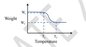
$W_i$  and  $W_f$  represent the weight of the material, corresponding to temperatures  $T_i$  and  $T_f$ , respectively. Which of the following factor(s) can influence  $T_i$  and  $T_f$ ?
